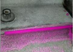
Barrier FS can also be applied to areas where product or water can easily accumulate. Apply while surfaces is relatively dry and monitor the rate at which it dissolves to determine repeat applications.
