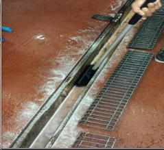
Scrub the drains with a designated black drain brush. Always follow the designated SSOP for drain and floor sanitation.
